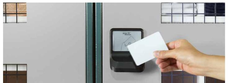
The textag lockers can be operated in stand-alone mode, or integrated into an existing access control system, so that staff can also use their personal access transponder for the texLocker. Access to the lockers can be administered individually for each user, or in groups. Only when the user has the appropriate access rights can the dispensing locker be opened to remove clothing.
